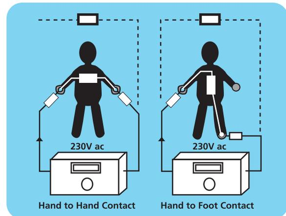
*Current passing through the body from one hand to the other or from hand to foot will pass through the chest area containing the heart and lungs.*
