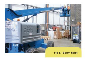
Work equipment used for lifting people must have a thorough examination, (e.g. see Figure 5) which should be carried out by a competent person at least every six months. Accessories for attaching to lifting equipment such as slings or chains must also be examined every six months. All lifting equipment must be inspected weekly by the owner or user and records of these and all examinations must be kept. Proper maintenance is also essential in ensuring that equipment is safe to use.
