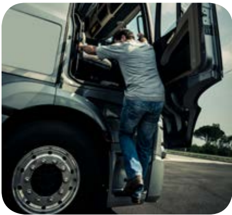
Figure 4: Three points of contact/ control on vehicle steps
