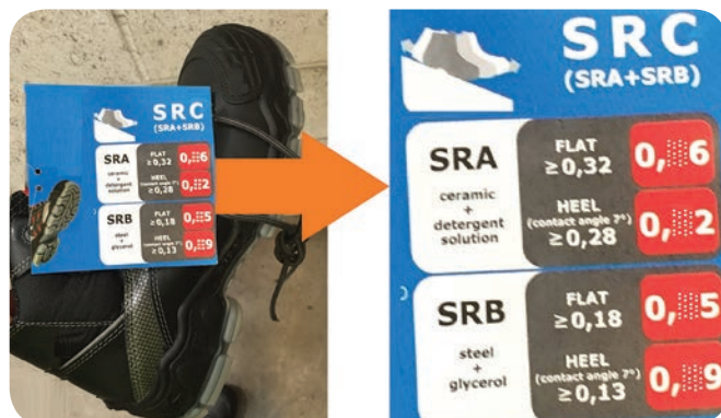
Figure 4. Label attached to footwear indicating slip resistance test results
