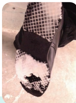
Figure 5. Clogged channels in slip-resistant footwear
