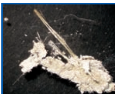
Amosite (brown asbestos) in Asbestos Insulating Board (AIB)
